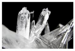
When you can no longer dissolve any more of the base material into the water, your solution is now a saturated solution. Cooling the solution quickly encourages rapid crystal growth, since there is less room for the dissolved salt in the cooler, denser solution.
